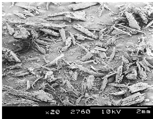
Figure 1. SEM micrograph of a 40 mesh wood flour sample.
